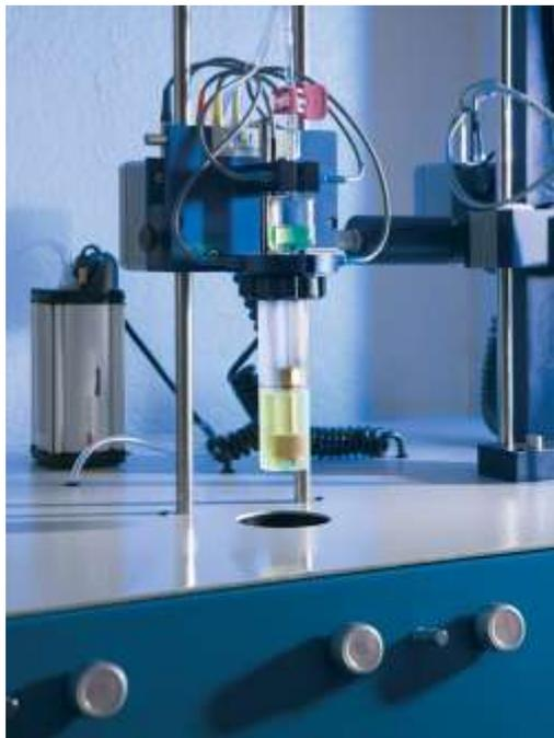
*A Cold-Filter Plugging Point (CFPP) test in progress.*
